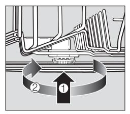
■ Lift up the <u>middle</u> spray arm b to engage the ratchet. Then unscrew the spray arm ②.
